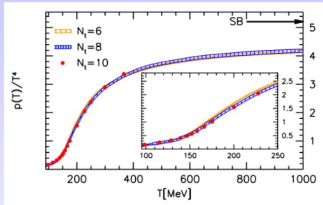
The pressure normalized by  $T^4$  as a function of the temperature on  $N_t=6,8$  and 10 lattices.
